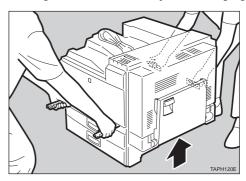
Push the grips into the printer. Take out the cover inside the Tray 2 and attach it between the paper tray and the front cover.
